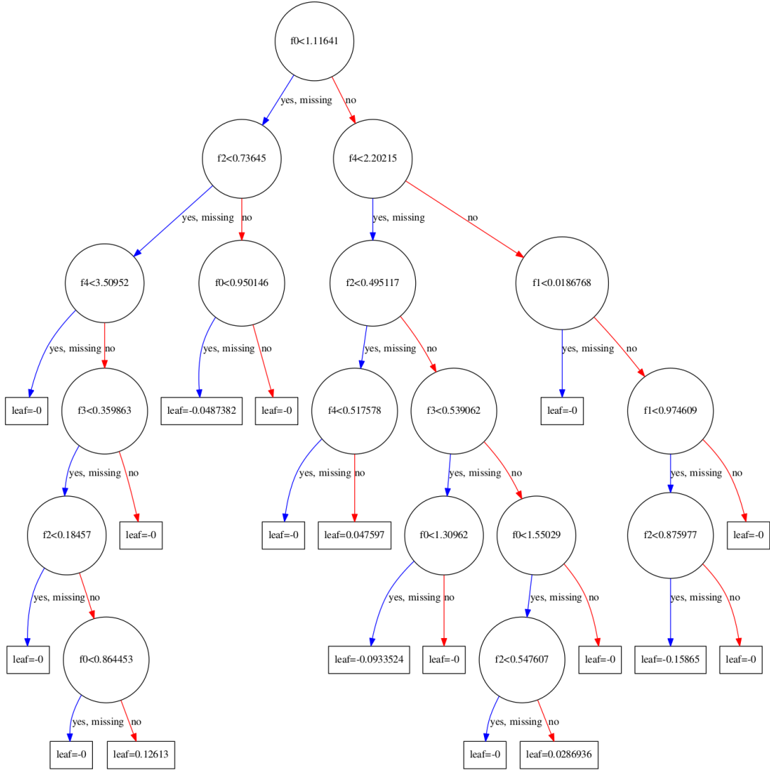
Figure 2: An example classification and regression tree (CART) used for regression. Features are labelled f_0, \dots, f_4 and nodes specify cutoff thresholds that designate the path a new parameter vector takes from the top (root) node to the final (leaf) node, which denotes the predicted calibration value. In the process of “boosting” CART trees to produce an ensemble, each subsequent tree increasingly focuses on the higher weighted samples. This generally results in smaller “specialized” trees that stick on samples that were most difficult to classify.
